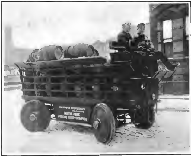
FRONT AND REAR WHEELS SET AT OPPOSITE ANGLES.
